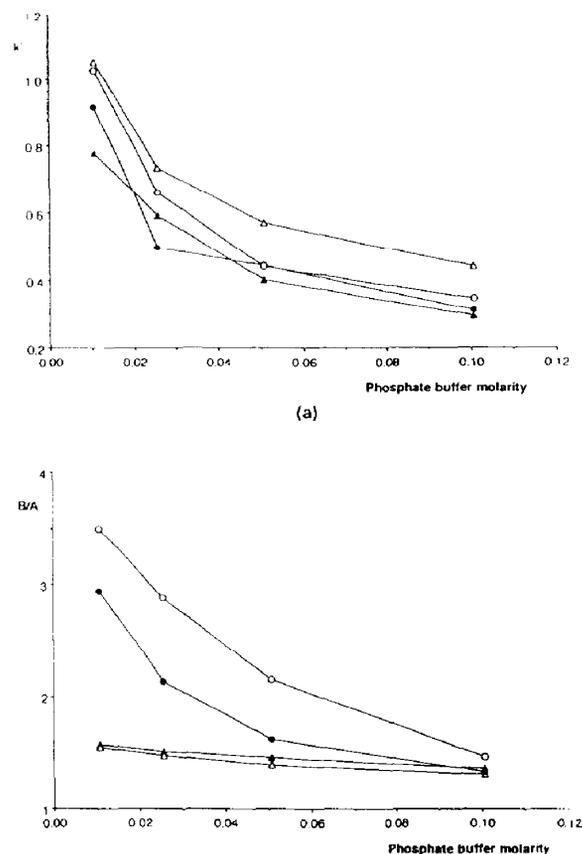
Fig. 1. Comparison of (a)  $k'$  and (b)  $B/A$  values vs. phosphate buffer concentrations with heptanesulfonate at two levels, from two stationary phases: RP-Select B and SGE 250 GL. Chromatographic conditions: mobile phase, methanol-buffer (50:50); flow-rate, 1 ml/min; detection, UV at 310 nm. ▲ = RP-Select B, 0.005 *M* HS; △ = RP-Select B, HS = 0.01 *M*; ● = SGE 250 GL, HS = 0.005 *M*; ○ = SGE 250 GL, HS = 0.01 *M*.
