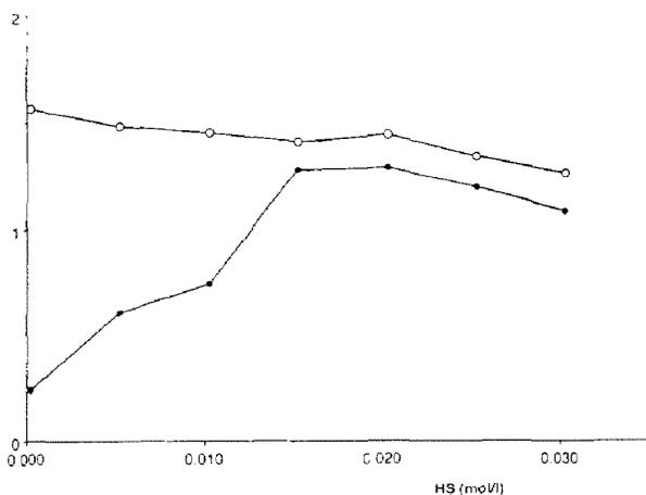
Fig. 2. Plots of (●)  $k'$  and (○)  $B/A$  vs. heptanesulfonate concentration of the mobile phase. Chromatographic conditions: column, LiChrospher RP-Select B; mobile phase, methanol–buffer (50:50), with  $2.5 \cdot 10^{-2}$  M phosphate buffer at pH 4.4.
