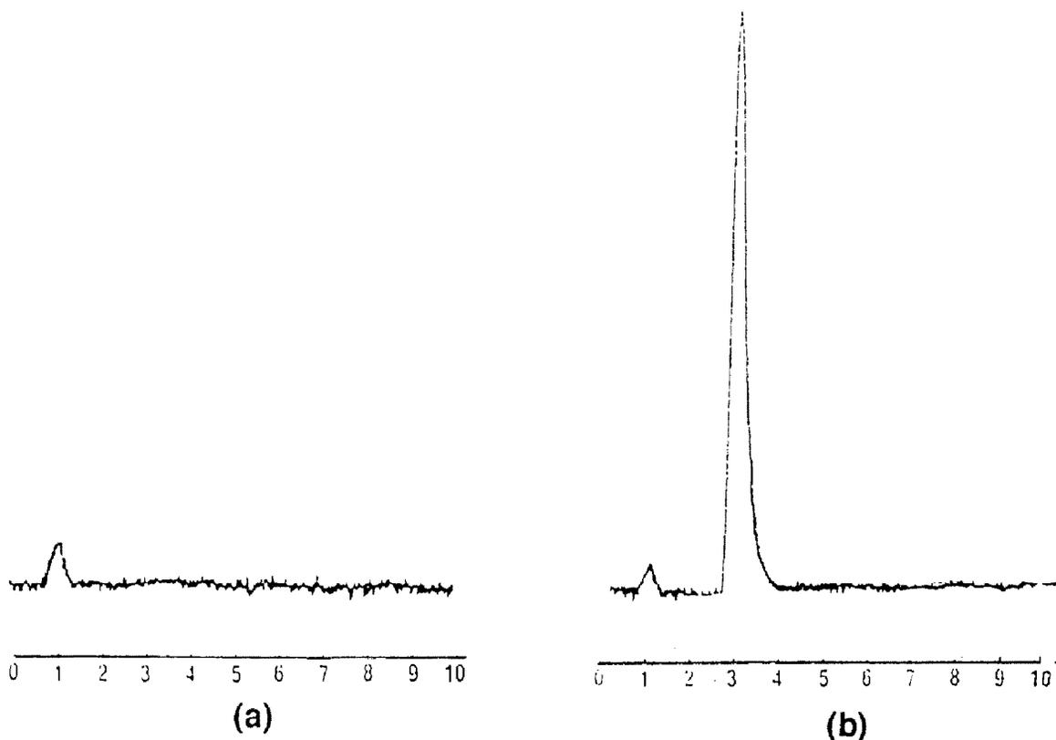
Fig. 3. Chromatogram of the components of the W/O/W multiple emulsion (a) without and (b) with dihydralazine. Chromatographic conditions: column, LiChrospher RP-Select B; mobile phase, methanol-buffer (50:50), with  $2.5 \cdot 10^{-2}$  M phosphate buffer at pH 4.4 and heptanesulfonate  $2.5 \cdot 10^{-2}$  M.
